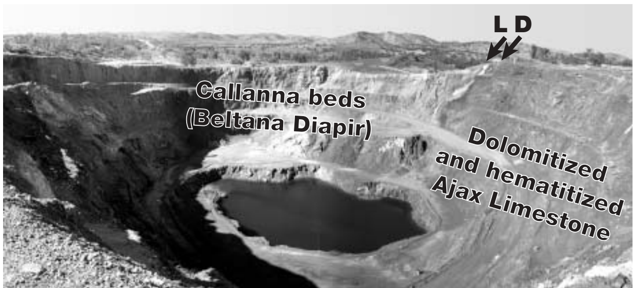
FIG. 10. View toward the south over the Beltana open pit. The arrows labeled L and D point to a quartzite lens (L) and a hematite-rich rock (D) that underline the contact between the Callanna beds and the Ajax Limestone.
