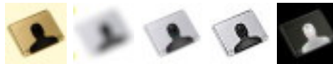
Figure 8: Tools for photographic picture transformation: sepia effet (1), smoothing (2), transformation to black and white (3), sharpening (4), color inversion (5) .
